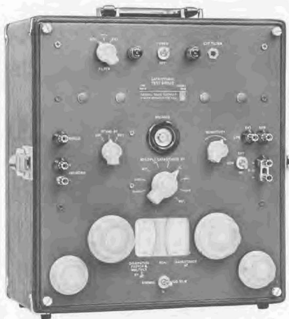
Figure 3. Current model of the Capacitance Test Bridge.
